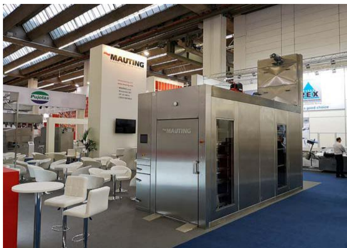
Fig. 4: The smoking and chilling chamber UKM/ZKM with a trolley transport system was in the visitor spotlight of the Mauting exhibition.
